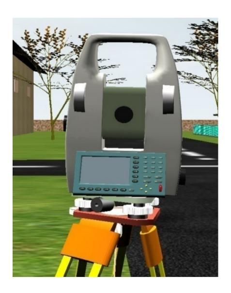
2. Fix the Total Station equipment over tripod. Level it and center it precisely over the ground point. (Use keys: Alt + Up, Down, Left, Right (Arrow Keys))
